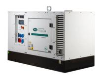
Ready-to-use power pack, complete with radiator, exhaust system, diesel fuel tank and dashboard. Operating speed 1500 rpm, single phase output 230 V 50 Hz, or 3 x 400 VAC, 50 Hz. 10 kVA power. Medium duty power solution.
