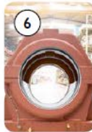
6 Intermediate shaftline bearing
