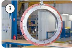
3 Fwd seal Oil lubricated
