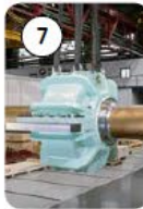
6 Intermediate shaftline bearing
