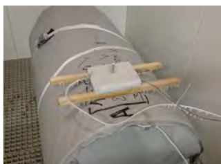
LIFERAFT STORED FOR 50HRS AT -70^{\circ}\text{C}
