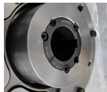
Taper lock bush on the hub of a flexible CT-H coupling
