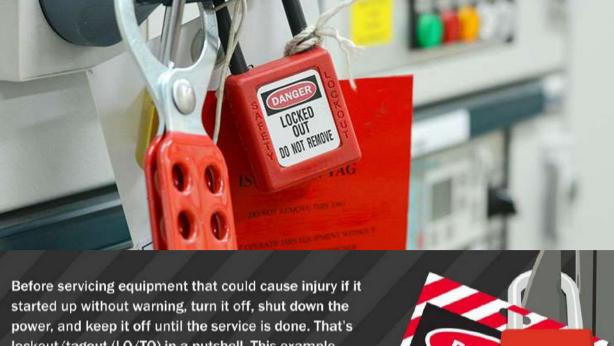
lockout/tagout (LO/TO) in a nutshell. This example sequence shows a step-by-step LO/TO process that can be easily adapted for any equipment in your facility. **LOCKING OUT EQUIPMENT**
