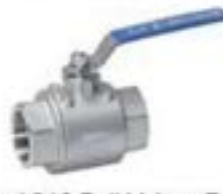
S.Steel 316 Ball Valves Full Bore 2 Piece Body Female Thread Ends
