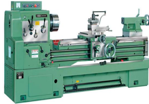
LATHE Milling MACHINE (2-axis / 580mm / 1350rpm)
