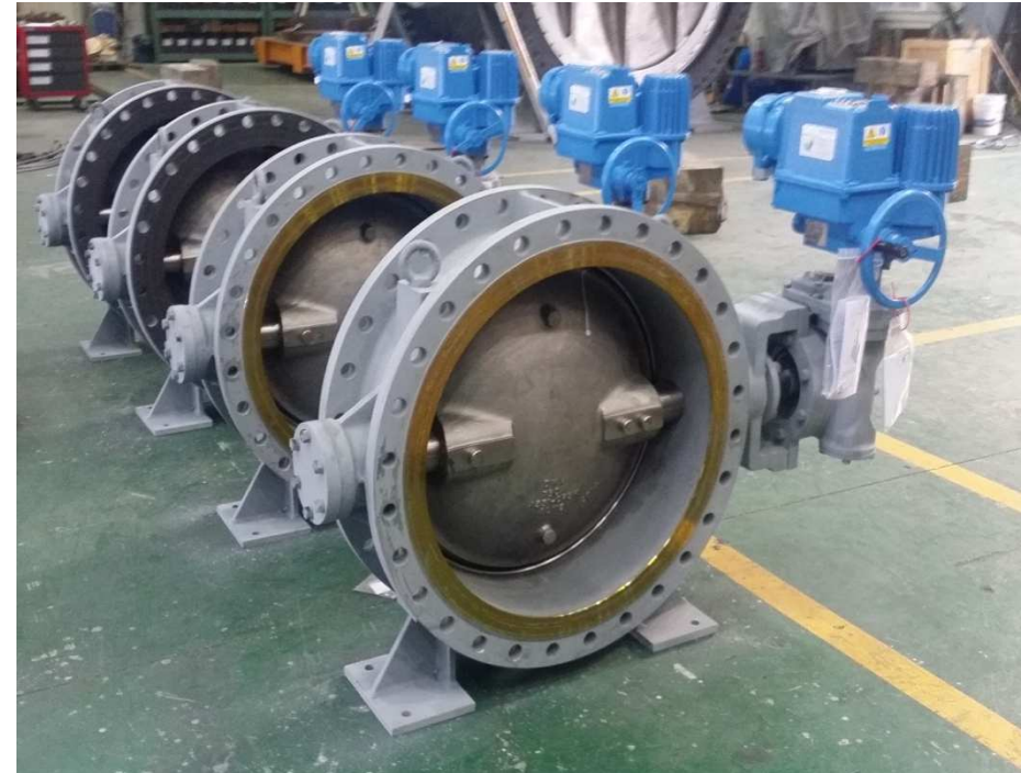
Motor Operated Butterfly Valve Size : 750A Project : Vietnam Thai Binh2 Thermal Power Plant Service : ACW PP Discharge Fluid : River(Brackish) Water
