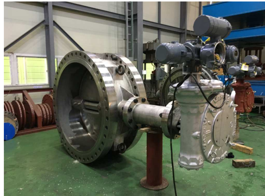
MOTOR OPERATED BUTTERFLY VALVE / METAL SEAT TYPE S-OIL RESIDUE UPGRADING COMPLEX PROJECT SIZE : 1500A #300 FLUID : HYDROCARBON(260℃)
