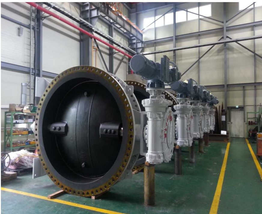
Motor Operated Butterfly Valve Size : 2200A Project : Taeon Thermal Power Plant Fluid : Sea Water
