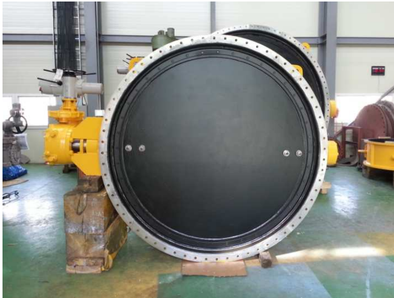
POSCO POHANG Gas Holder Main Line 3400A Fluid : LDG
