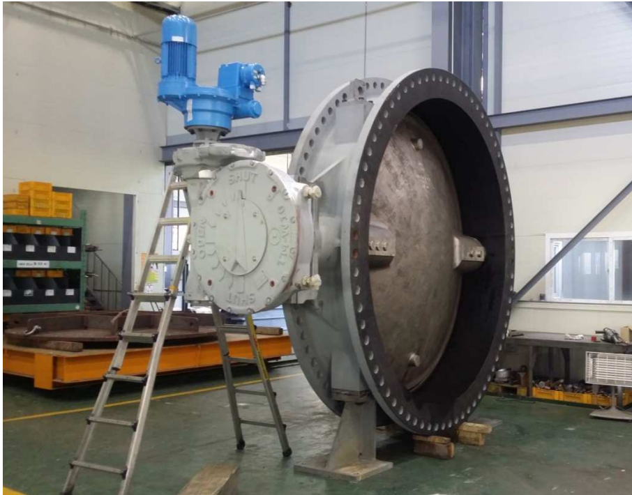
Motor Operated Butterfly Valve Size : 2700A Project : Vietnam Thai Binh2 Thermal Power Plant Service : CWP Discharge Fluid : River(Brackish) Water
