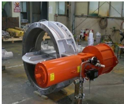
PNR PLANT/ NSCE/POSCO Control/Shut-off VALVE Design Temp: -30~ 450 °C Size : 50A~ 1500A
