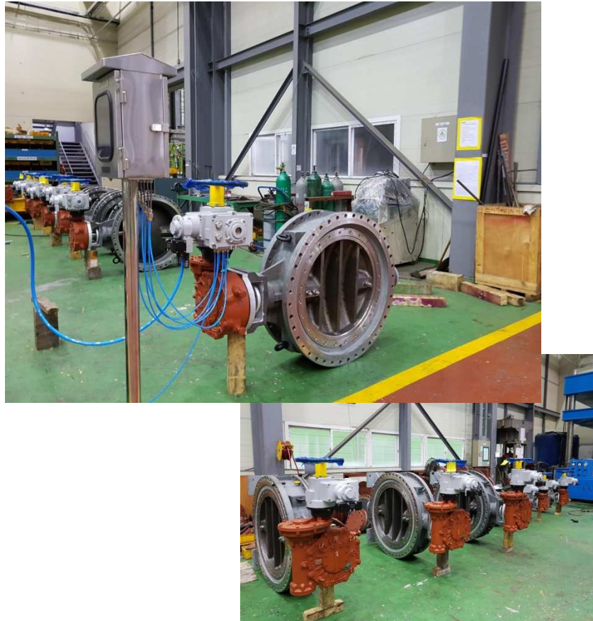
AIR MOTOR OPERATED BUTTERFLY VALVE / METAL SEAT TYPE S-OIL RESIDUE UPGRADING COMPLEX PROJECT SIZE : 300A,400A,650A,850A,1000A #150 FLUID : COOLING WATER/PROPYLENE OXIDE(LIQUID)
