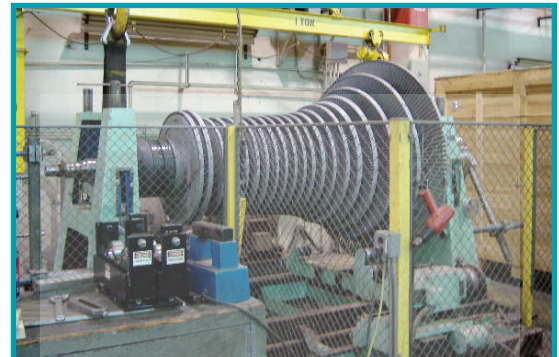
Dynamic balancing of a 10 MW turbine rotor
