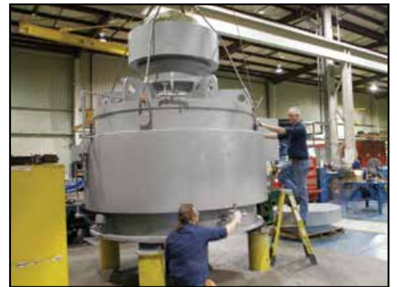
Circulating Water Pump Motor: 2,500 HP, 6,600 V, 52,000 lbs.
