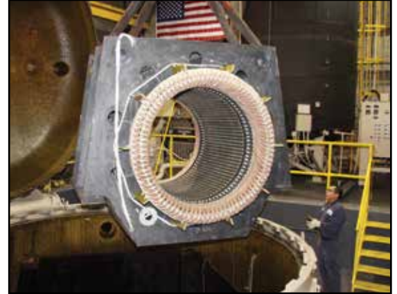
Main Compressor Motor: 22,500 HP, 13.8 kV, 35,000 lb. stator
