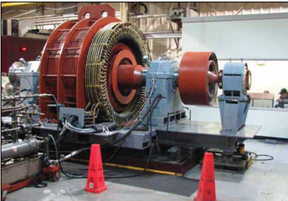
Main compressor synchronous motor (15,000 HP, 13.8 kV, 96,000 lbs.) on test. Test stand is capable of no-load tests up to 37,500 HP and load tests up to 4,500 HP - both at 15 kV.
