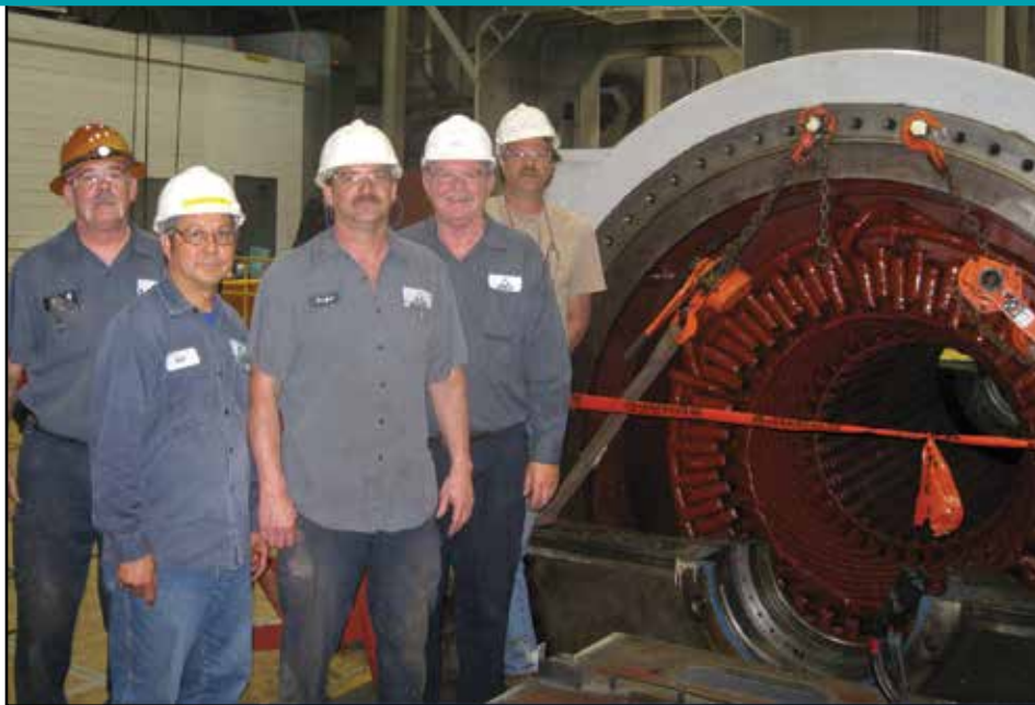
IPS field service technicians work on a 44 MW GE hydrogen-cooled generator.
