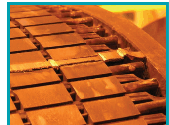
Broken rotor bar
