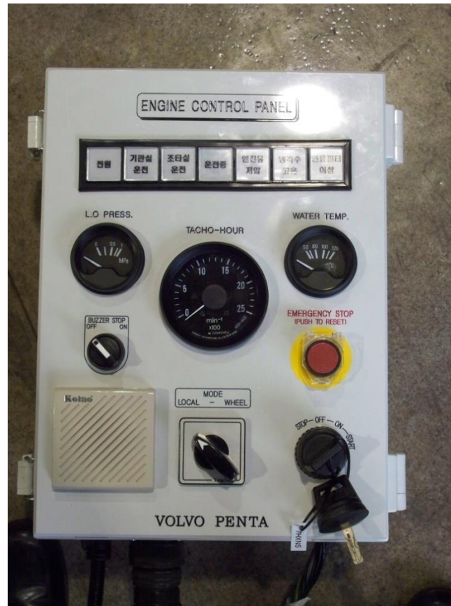
ENGINE CONTROL PANEL
