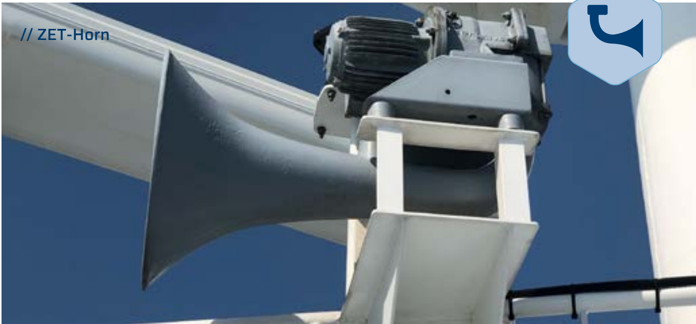
Fig. top ZET-Horn 131 AC is on daily duty when crossing the Elbe on the pilot vessel.
