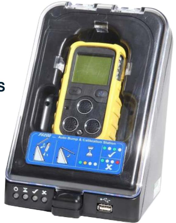
The MED approved ABC™ system delivers on-board automatic and fail-safe calibration and bump testing of your detectors during re-charging. The equipment automatically generates a tamper-proof serial number, specific calibration certificates which are free from human intervention and error.
